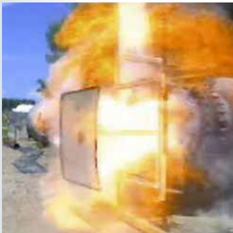
Vented Dust Explosion: 6 pounds of Corn Starch ignited in a 100 cubic foot test vessel
