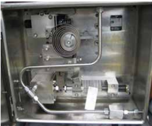
BPIV Buckling Pin Mechanism (Closed Position)
